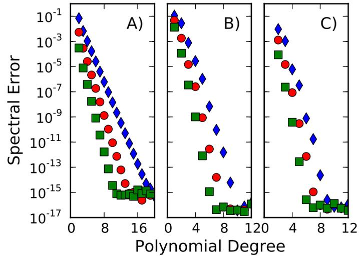
Figure 4: Spectral error in  $\psi$  for the A)Solev'ev equilibrium, B)FRC equilibrium, and C) spheromak equilibrium for a 2x2 ( $\blacklozenge$ ), 4x4 ( $\bullet$ ), and 8x8 ( $\blacksquare$ ) element mesh.
