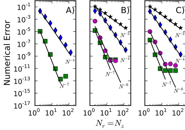
Figure 2: H-refinement convergence studies for the A)Solev'ev equilibrium, B)FRC equilibrium, and C) spheromak equilibrium. The numerical error in  $\psi$  is plotted for 2nd order elements ( $\blacklozenge$ ) and 6th order elements ( $\blacksquare$ ). The numerical error in  $B_r$  is also plotted for the FRC and spheromak equilibria for polynomials of degree 2 ( $\star$ ) and polynomials of degree 6 ( $\blacklozenge$ ). Reference lines are added showing indicated rates of convergence.
