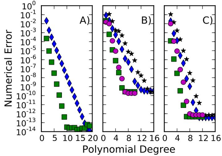
Figure 3: P-refinement convergence studies for the A)Solev'ev equilibrium, B)FRC equilibrium, and C) spheromak equilibrium. The numerical error in  $\psi$  is plotted for a 2x2 ( $\blacklozenge$ ) and 8x8 ( $\blacksquare$ ) element mesh. The numerical error in  $B_r$  is also plotted for the FRC and spheromak equilibria for the 2x2 mesh ( $\star$ ) and 8x8 ( $\bullet$ ) element mesh.
